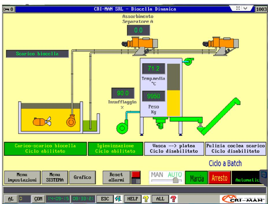
The main page of the management software displays all the components of the HBC separation system with continuous updating of the process data (temperature, weight, air input)
